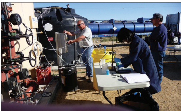
Left: The regeneration team and researchers collect water samples from tank B during the regeneration process. Right: Regeneration team members prepare the caustic regeneration solution in the storage tank.
